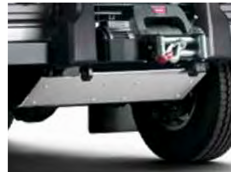
Mudflaps RTC9479 Heavy duty moulded mudflaps reduce spray and help protect vehicle paintwork. Mudflaps, front pair for 90 and 110 models only.
